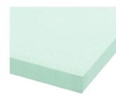
Claylite is a low density expanded polystyrene compressible-fill material which can be used to reduce the pressure exerted on reinforced concrete ground beams or on the vertical face of concrete foundations.
