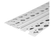
PVC Movement Beads are used to accommodate movement in plaster, stucco, or render finishes. It helps prevent cracking in large or long sections of walls or ceilings by allowing for controlled expansion and contraction.
