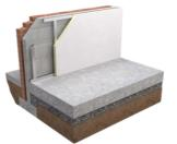
Thin-R Thermal Liner is a composite insulated panel of Unilin PIR insulation core with a composite foil facing bonded to 12.5mm tapered edge plasterboard for internal walls, sloped roofs, and ceilings.
