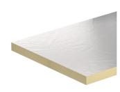
Thermaroof TR26 is a PIR, flatroof insulation board, offering a thermal conductivity of 0.022 W/mK. It is fully compatible with most mechanically-fixed, single-ply waterproofing systems and most green roof systems.
